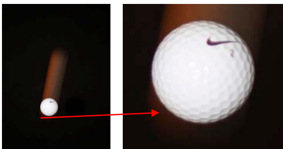
Fig 1A - Canon Rear Curtain Sync - note leading edge of the motion blur. 1D mk III camera used for example.
